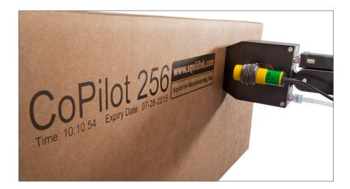
1) The CoPilot 256 utilizes oil-based, solvent-based, or UV curable inks for printing on a wide range of porous or non-porous substrates.
